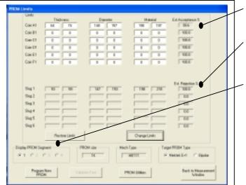
For Coin A1 the Limits generated for each parameter are shown along with the Estimated Acceptance %age (based on the coins used for programming)
